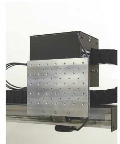
Left image - probe head assembly with Z axis probe head and camera mounted Right Image - special adapter plate that allows for complete head customization
